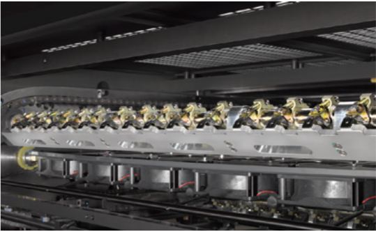
Gripper shaft Stable sheet transport is achieved by the shape of the gripper shaft, which was determined through air simulation. Improves sheet alignment.
