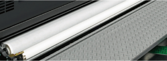
Automatic impression cylinder cleaning*
